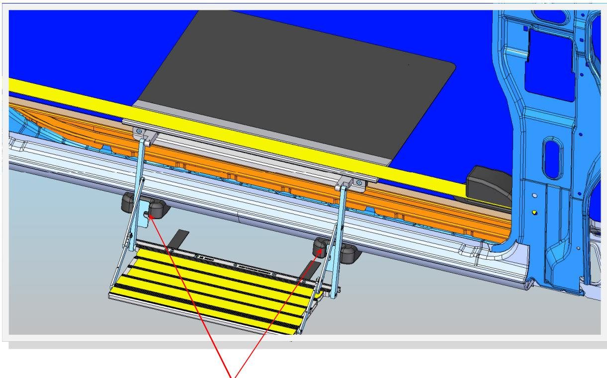
**Note: The drop arm plates *MUST* locate in the black plastic Guide Blocks as shown.**
